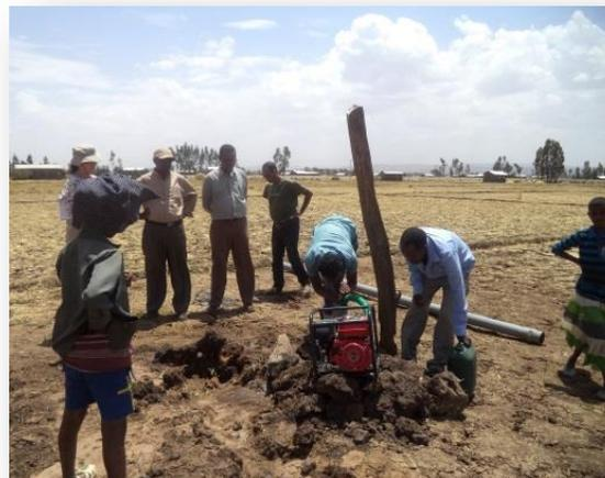
motor pumps used for irrigation.
